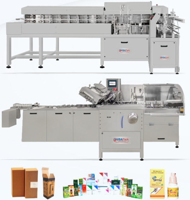
Semi-Automatic & Automatic Cartoning Machine with Output Speed 50 PPM to 300 PPM
